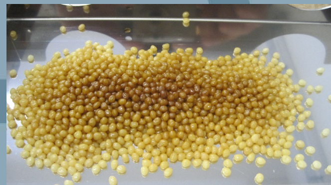
Material burns or oxidates due to an over drying
